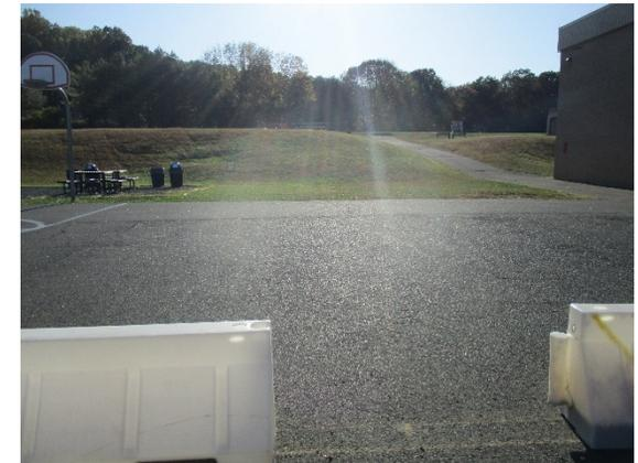
Two rain gardens can be installed adjacent to the entrance of the building and in the turfgrass south of the building to capture, treat, and infiltrate rooftop runoff. A section of parking spaces can be converted to pervious pavement to capture and infiltrate stormwater. A preliminary soil assessment suggests that more soil testing would be required before determining the soil's suitability for green infrastructure.
